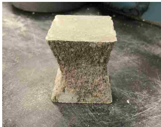
Figure 3-4: Mortar Cube After Compression Testing
