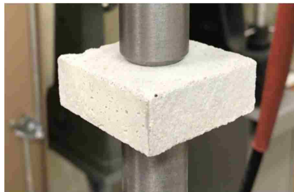
Figure 3-8: Mortar Specimen Tested with the Double Punch Test
