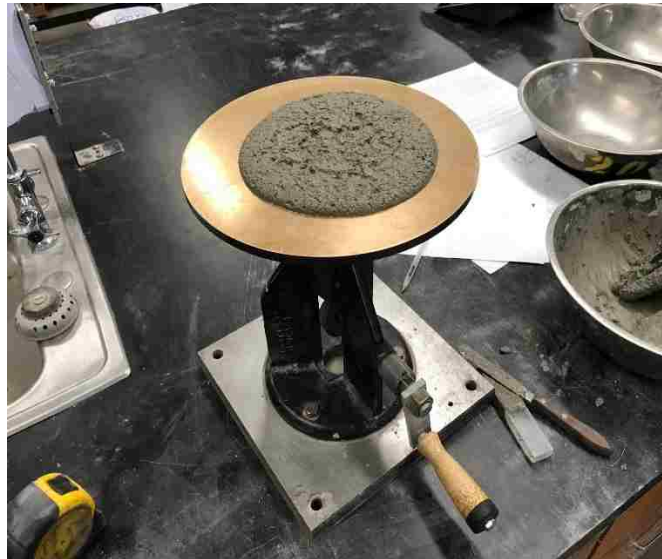
Figure 3-1: Mortar Flow Test
